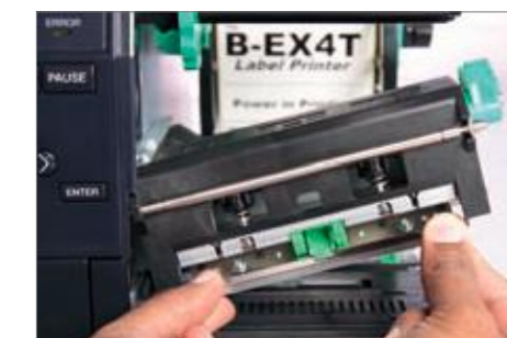
Snap-in printhead reduces maintenance downtime to a minimum
